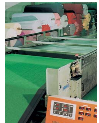
Cross-lapping of web layers in the nonwoven industry. High production speed and acceleration of masses while the web is guided directly between the belts places extremely high demands on the processing belts.
