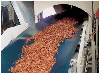
Horizontal conveying with troughable belts. The tension member construction provides the flexibility in the desired direction.
