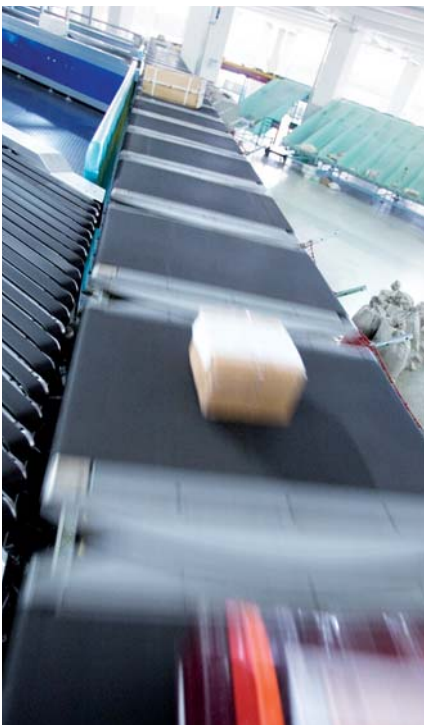
Lateral sorter in a distribution centre. The high acceleration requires the belt surface to have an extremely high coefficient of friction.
