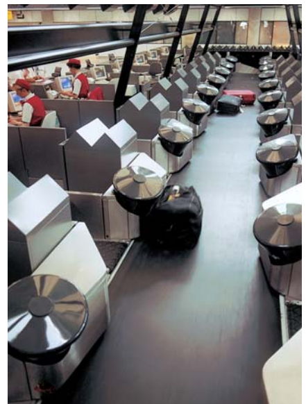
Collecting belt in check-in area of an airport. The flatness of the belt type here ensures that the goods can be discharged to the side smoothly, even on wide belts. Flame-retardance is a "must" in modern airports.
